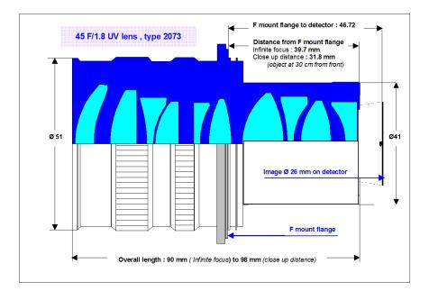
The **45 F/1.8 UV lens type CERCO® 2073** has been designed for intensified CCD video cameras with UV photocathode (diameter 18 or 25 mm). This UV lens achieves the best luminous efficiency for ultraviolet imaging, thanks to its F/1.8 aperture and multilayer antireflective coatings.
