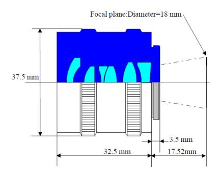
The **28 F/3.5 UV lens type CERCO® 1990** has been designed for video cameras with image intensifier working with UV light. This UV lens is usable from ultraviolet to near infrared without focusing adjustment. Two types are proposed: standard multicoated type, optimised from 240nm to 410 nm wavelength range, and uncoated type, usable from 190 nm to 900 nm.
